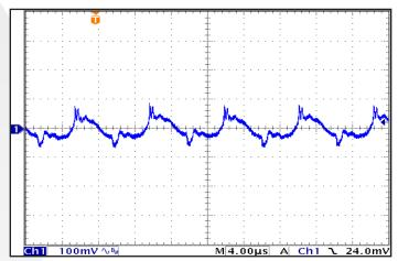
Figure 10: Output Voltage Ripple, Vout, at nominal input voltage and rated load current (100 mV/div). Load capacitance: 1μF ceramic capacitor and 100μF electrolytic capacitor. Bandwidth: 20 MHz. See Figure 13.
