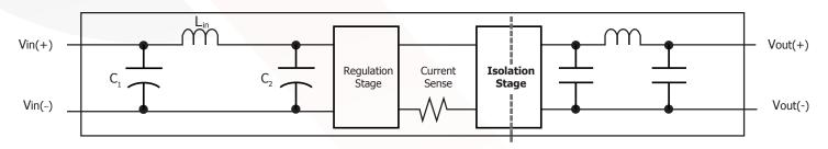
Figure E: Internal Input and Output Filter Diagram (component values listed in Electrical Characteristics section)
