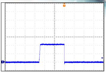
Figure 14: Output Short Load Current (20A/div) as a function of time (20ms/div) when the converter attempts to turn on into a 1 m $\Omega$  short circuit.
