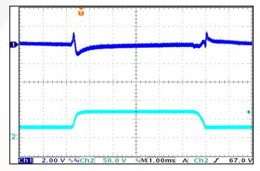
Figure 12: Output Voltage Response to Step-Change in Input Voltage (250V/ms). Load cap:  $100 \mu F$  electrolytic output capacitance. Ch 1: Vout (2V/div), Ch 2: Vin (50V/div).
