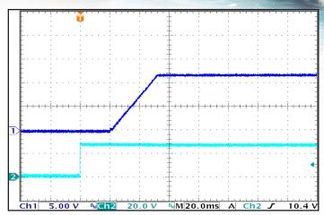
Figure 8: Turn-On Transient at full resistive load and zero output capacitance initiated by Vin. Ch 1: Vout (5V/div). Ch 2: Vin (20V/div).
