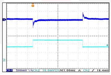
Figure 11: Output Voltage Response to Step-Change in Load Current (50%-75%-50% of Iout(max); dI/dt=5 A/ $\mu$ s). Load cap: 1  $\mu$ F ceramic and 100  $\mu$ F electrolytic capacitors. Ch 1: Vout (500mV/div), Ch 2: Iout (10A/div).
