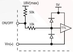
Figure B: Internal ON/OFF Pin Circuitry
